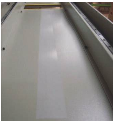
1. Stick a layer of PTFE on the workbench in contact with the cable chain.
